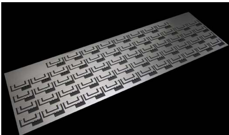
Fig. 2. Sheet of hinges formed on the punch press using Mate hinge tooling. Secondary forming operations and tooling eliminated.
