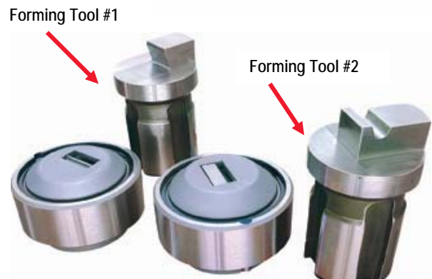
Fig. 1. Hinge forming tools, shown in 114-Style tooling.
