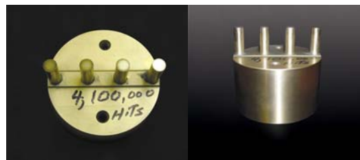
Photos of the actual Maxima treated tool that racked up over 4.1 million hits without sharpening.
