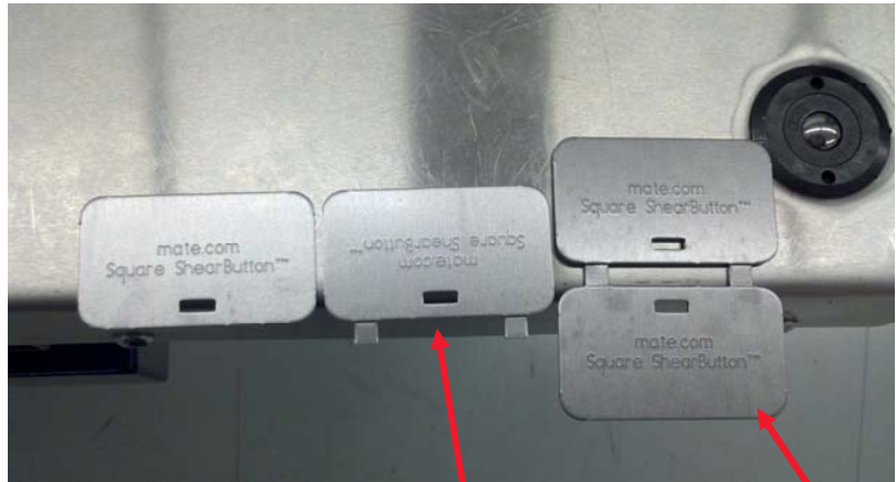
Square ShearButton shown after punching and ready to be removed, before separating parts after removal from sheet.
