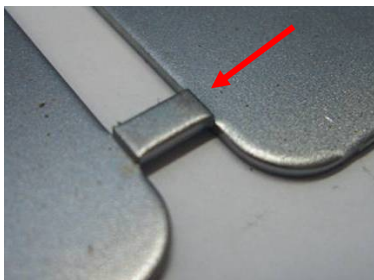
Above photo shows the snap line created with the Square ShearButton tool.
