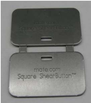
Square ShearButton example, before separating parts. Note: 2 tabs shown, but 1 tab would be plenty strong.
