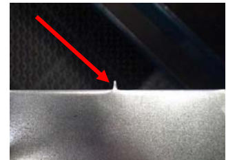
Example of the burr left over as the result of a wire joint process.
