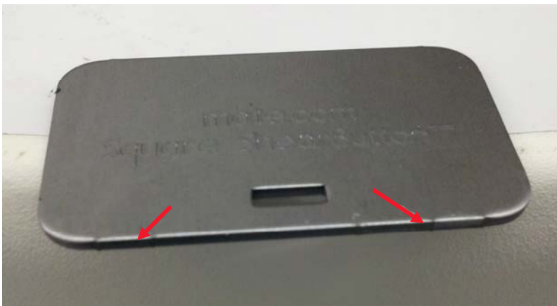
Square ShearButton (form down) after removal from sheet shows smooth edge quality.
