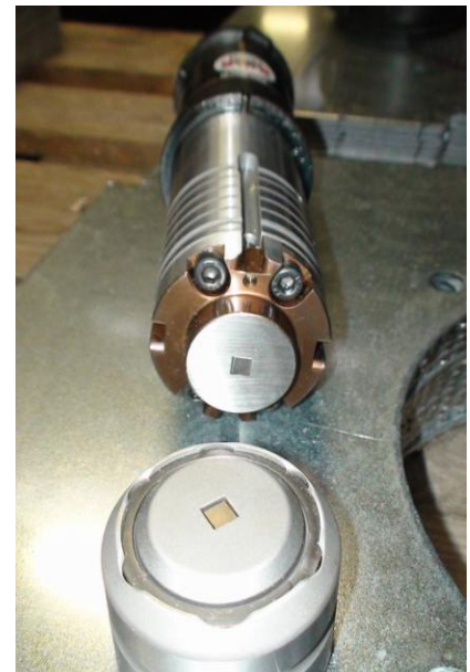
Square ShearButton in Ultraform holder.
